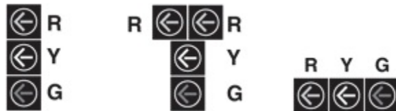
(b) Typical Signal Head Arrangements for Fully Protected LTs
