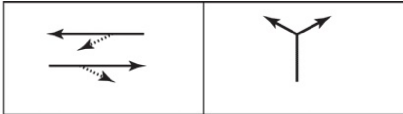
(a) A Two-Phase Signal Plan for the T-Intersection of Figure 17.9 (Permitted Left Turns)
