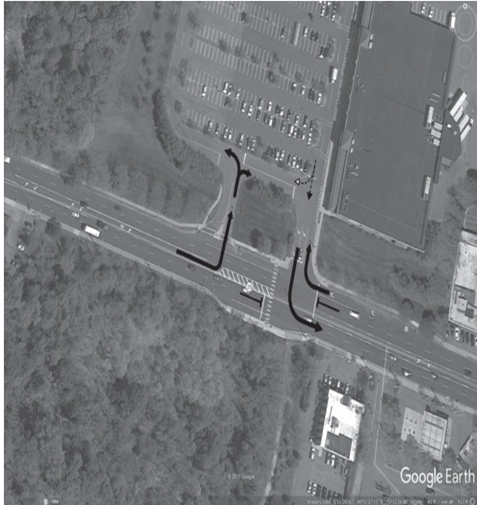
(b) Left Turns on One Phase, Thru Traffic on Another Phase
