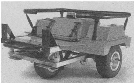
Figure 6-14. GripTester Surface Friction Tester (Findlay, Irvine Ltd 2004).
