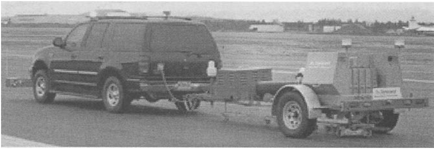
Figure 4-2. Heavy Dynatest FWD (HWD).
