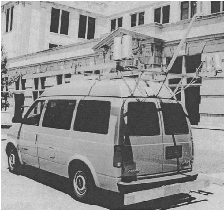
Figure 3-37. Digital Camera Data Collection Vehicle (Cline et al., 2001)
